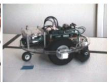
The Ebot is a differentially steered circular platform, with modified R/C servos providing the motive power. While quite functional, many members expressed a desire to have a platform that utilizes geared DC motors instead of servos, and provides room for adding upgrades such as wheel encoders, range sensors, bump skirt switches, etc.
