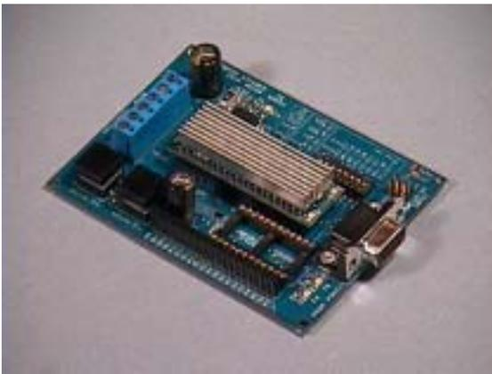
3.) The MMC is installed in the J2 DIP socket, with the LEDs closest to the serial connector. Place the carrier board on a firm surface, and align the MMC pins with the socket before pressing firmly on the heat sink. Be sure the MMC is seated all the way around.
