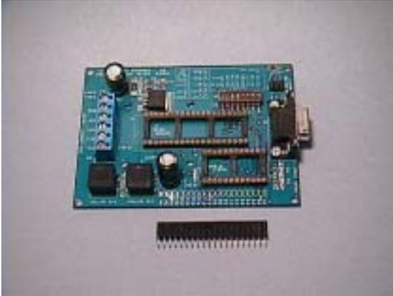
1.) The MMC carrier board has provisions for accessing the individual micro controller pins via solder connections at J6. Since the board would be used as a robot controller, a .100 mil 20 pin single row receptacle was added to J6 to make for easy connections.
