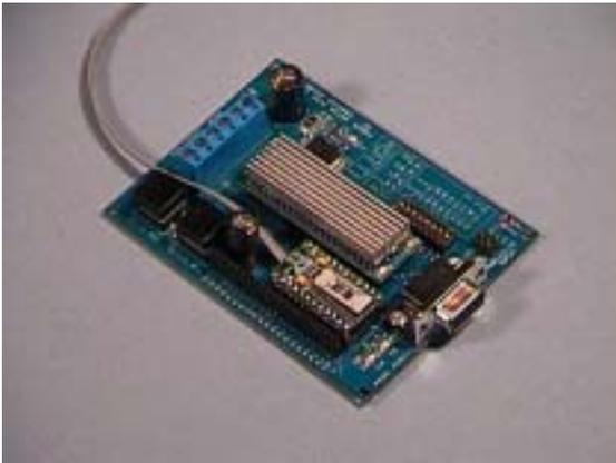
4.) The ATOM microprocessor is installed in J4 DIP socket. Exercise care when seating the ATOM's pins. The gray ribbon cable coming from underneath the ATOM in this photo was added prior to installation. The four conductors are soldered to the A0–A3 solder pads on the underside of the ATOM, which are used for A to D input.
